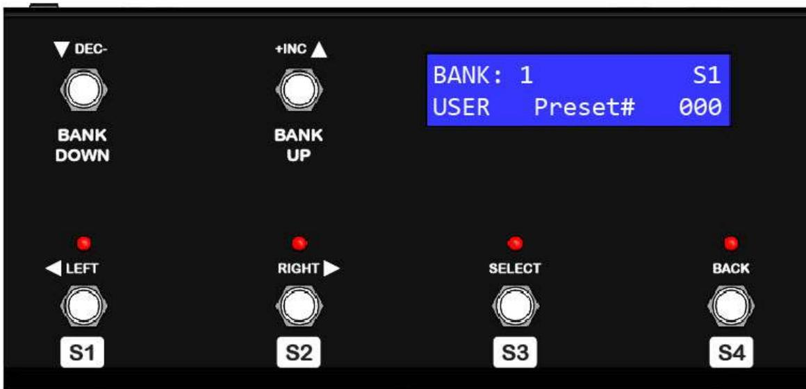
**BANK UP/DOWN SWITCH:** This is used to increase the bank up or decrease the bank down from the current state. The current bank starts from bank#1 up to a maximum of bank#32. You also use these switches in programming mode to edit parameter inside the menu selection.
